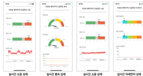
Screen displaying integrated measurement of wind, noise and fugitive dust in the field
